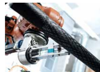
Automated winding process for manufacturing carbon fibre reinforced lightweight parts. Image: Peak Technology GmbH
