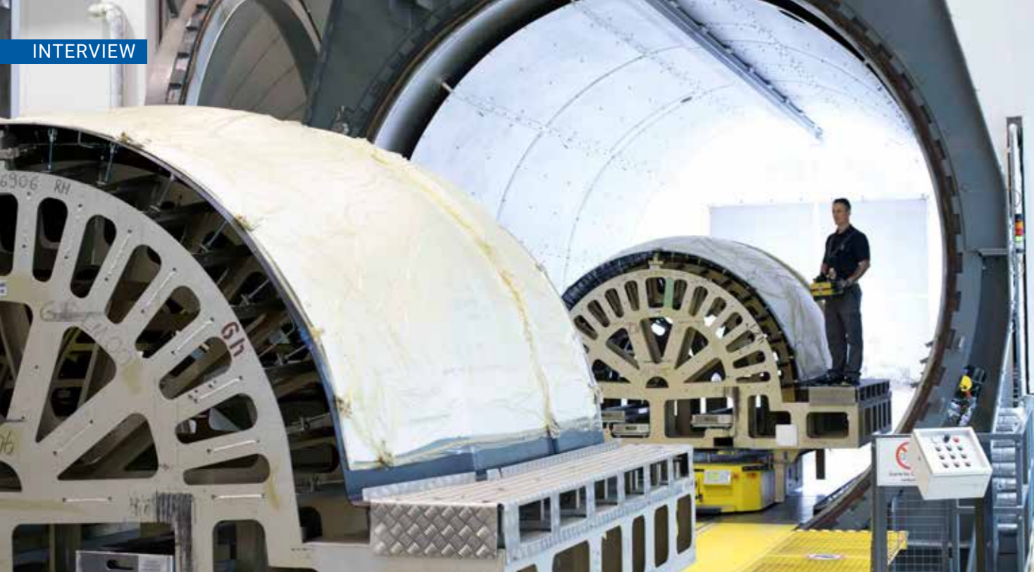
Among other things, FACC produces fairings and components for aircraft engines. Image: FACC/Bartsch
