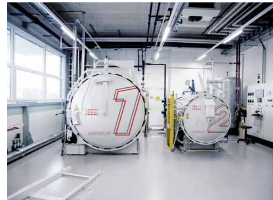
Wound and laminated parts are cured under pressure in the autoclave. Image: Peak Technology GmbH
