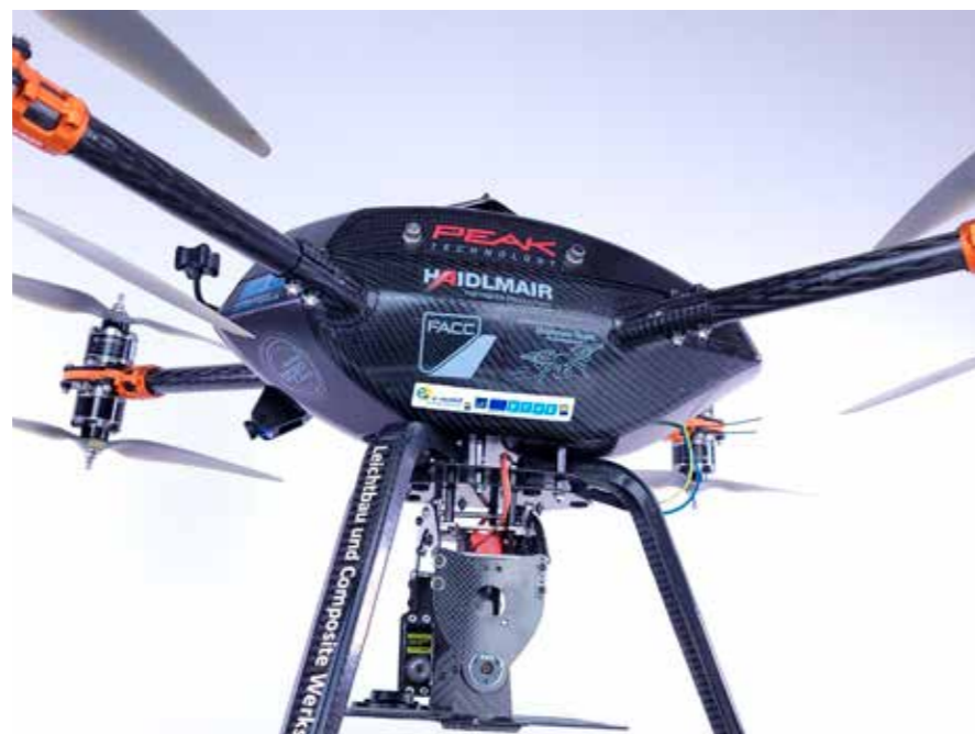
Weight-saving, high-strength composites are the ideal material for drones. Students at the University of Applied Sciences Upper Austria applied their know-how and expertise in lightweight design to develop a camera drone in a very integral design and enable a weight saving of more than 40 %. Image: FH 00
