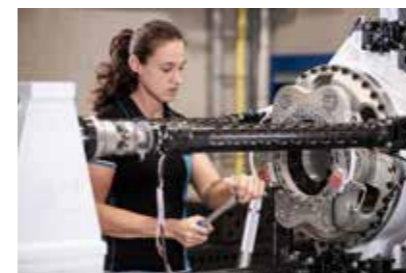
Validating lightweight components on the engine and drivetrain test beds. Image: Pankl Racing Systems AG
